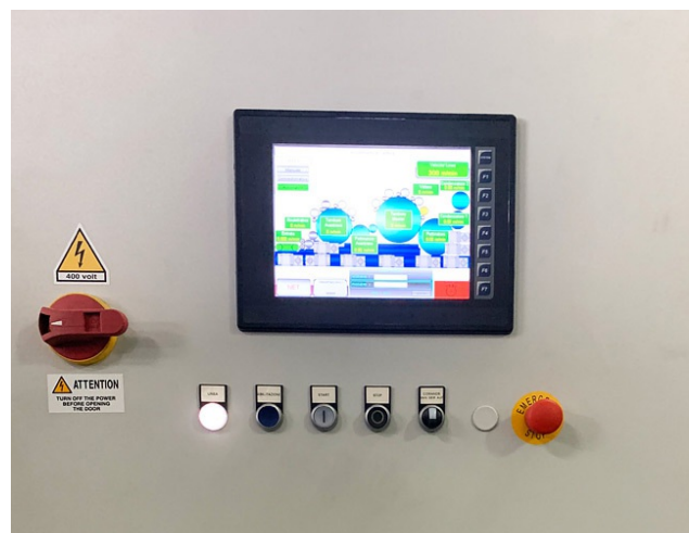
The eXL10 programmable logic controller and human machine interface device in the machine's cabinet (Source: Horner)
